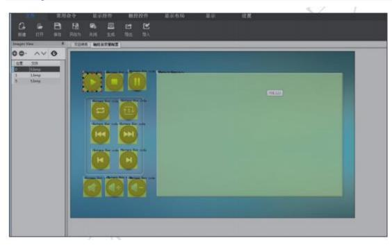
2. On the page of 0.bMP, select [Key Return] in the touch control and select the location to play in the figure. In the property setting, the variable address is: 0510 and the key value is: 5A00.Complete the playback control Settings.
