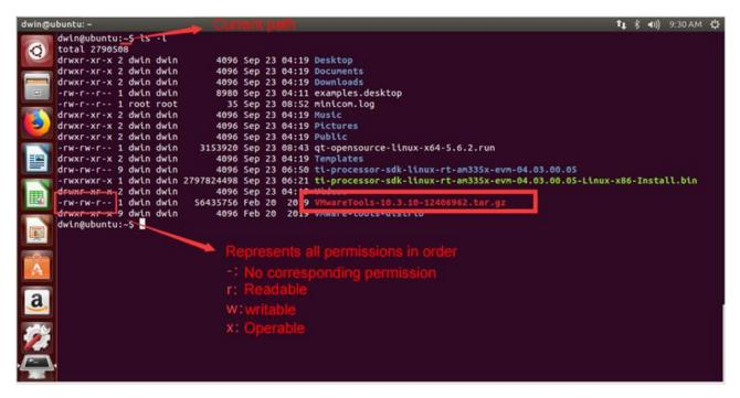
(8) Enter the command to enable the operable privilege: **sudo chmod +x VM** (to display the full name by **Tab** key) (**enter**), then enter the command: **Is -I (enter)**, and then you can see the target file become a green operable file. (Note: for the first time to use the administrator sudo privilege, you need to enter the password, i.e., the login password, which is not visible when entering.)
