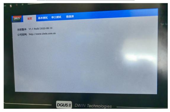
Note: touch screen may not work because of the lack of the configuration of the environment variable. Reboot and you can configure the environment variable refer to /etc/init.d/rcS.
