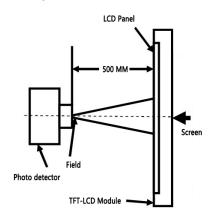
Note 2: Definition of viewing angle range and measurement system. The viewing angle is measured at the center point of the LCD by BM-7A.
