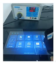
3.1 Electrostatic discharge test
